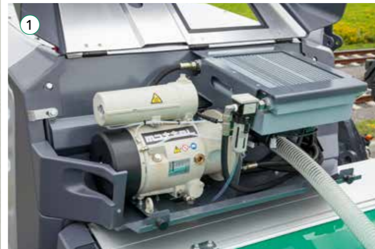
1 The spray nozzles are opened and closed pneumatically. A compressed air system is integrated in the SprayJet module for this purpose.
