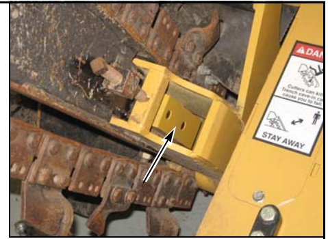
Optional backfill blade spacer assembly
