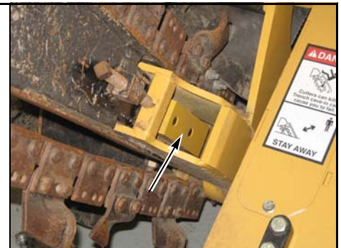
Optional backfill blade spacer assembly
