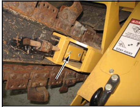
Standard block installed at factory
